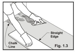
1.3 Spread only as much adhesive as can be used during open time of adhesive (Fig. 1.3).
